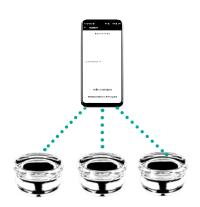
Grouping: possibility to create groups of Crystal Studs PLRE2 on the application and to control them simultaneously.
